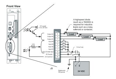
Figure 18: Epsilon Input/Output Wiring Diagram
